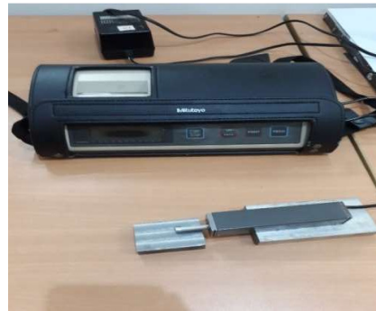
Figure 2. The surface roughness measuring of a specimen
