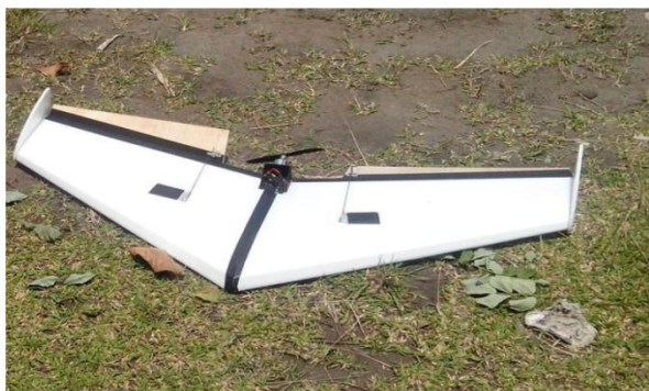
Gambar 2. Contoh UAV tipe flying wings [6]
