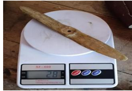
Figure 5. Finished propeller made from mother-in-law's tongue fiber.
