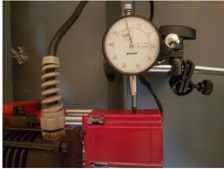
Figure 25. The third calibration result for the Z-axis stepper motor – DTI
