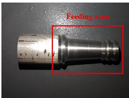
Figure 30. The results of the workpiece feeding for the second workpiece design – aluminum
