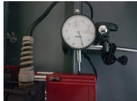
Figure 21. The first calibration result for the Z-axis stepper motor – DTI
