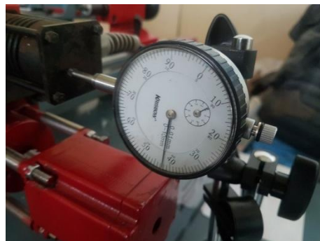
Figure 15. The first calibration result for the X-axis stepper motor – DTI
