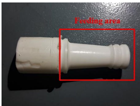
Figure 29. The results of the workpiece feeding for the second workpiece design – Teflon
