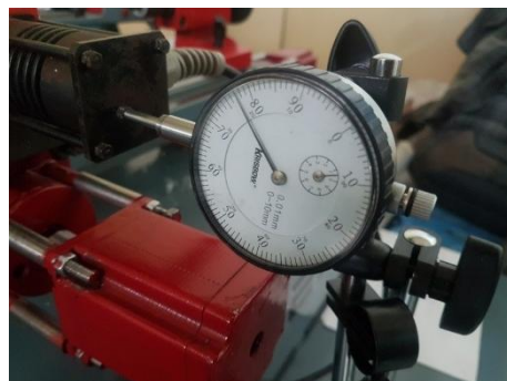
Figure 17. The second calibration result for the X-axis stepper motor – DTI
