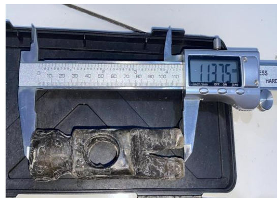
Figure 10. Mold Design Dimensions and Measurement Methods
