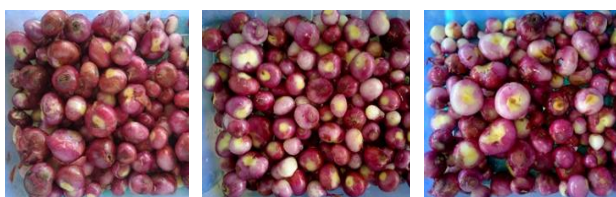
(a) Peeling results for 1.5 minutes (b) Peeling results for 2 minutes (c) Peeling results for 2.5 minutes
