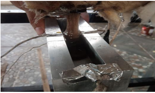
Figure 8. Injection of plastic liquid into plastic beam mould (barrel temperature 160°C)
