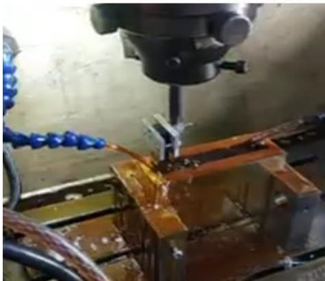
Figure 7. Mould electrical discharge machine (EDM) process
