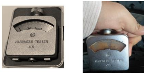
Figure 3. Measuring tire hardness using durometer
