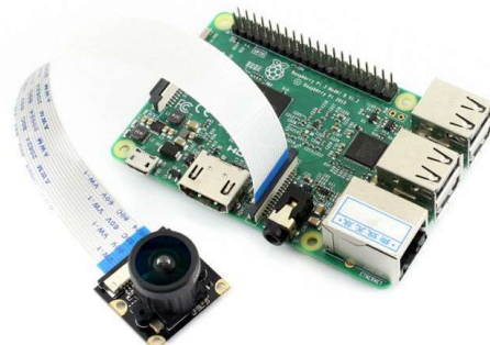
Figure 4. Raspberry Pi and camera module connection
