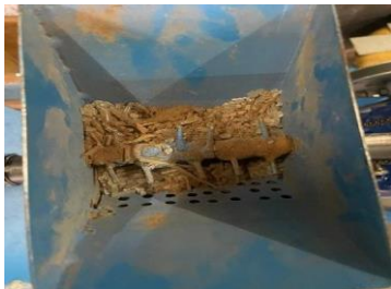
Figure 6: Put the material in the hopper
