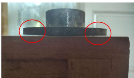
Figure 3. Cover existing lower dies on a flat surface by displaying different sides to show clarity (in red circle)
