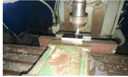
Figure 1. The milling process of making a specimen.
