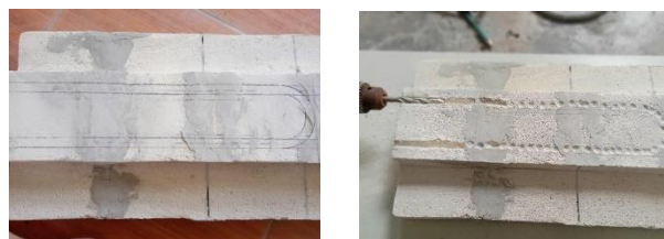
Figure 8. The line manufacturing process for heating coils
