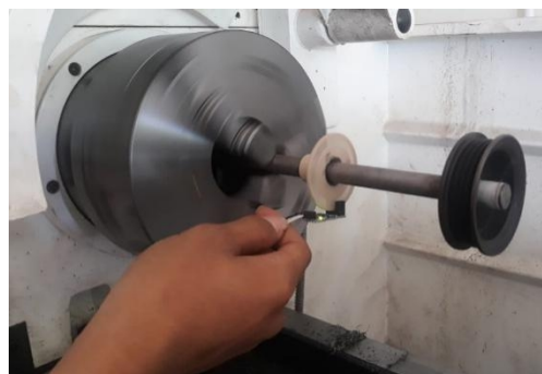
Gambar 12. Proses Kalibrasi IR LM393 Speed Sensor
